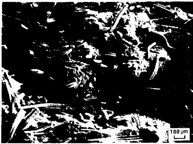
Fig. 5 SEM photograph of tensile fracture surface of composite containing 40 wt % nickel fibres of length 1000 µm
